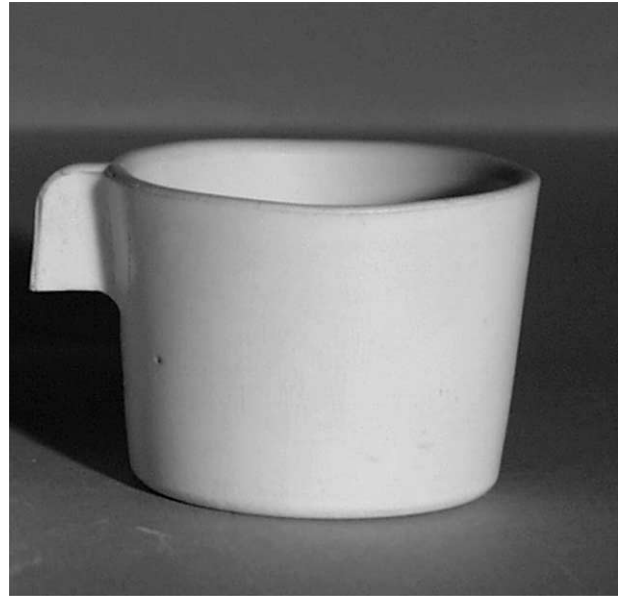
Fig. 10. Picture of a sintered porcelain cup obtained by aqueous injection moulding.
