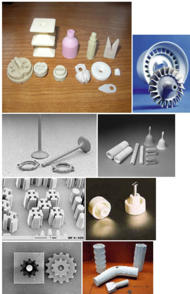
9 Ceramic components produced by low pressure injection moulding technology
