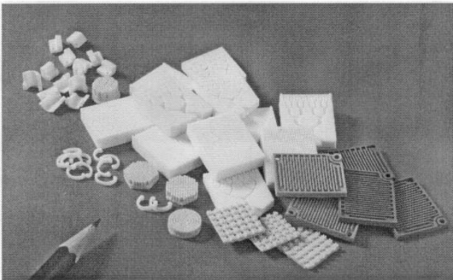
Figure 3. Microcomponents made of different ceramic materials fabricated by the RPPC.
